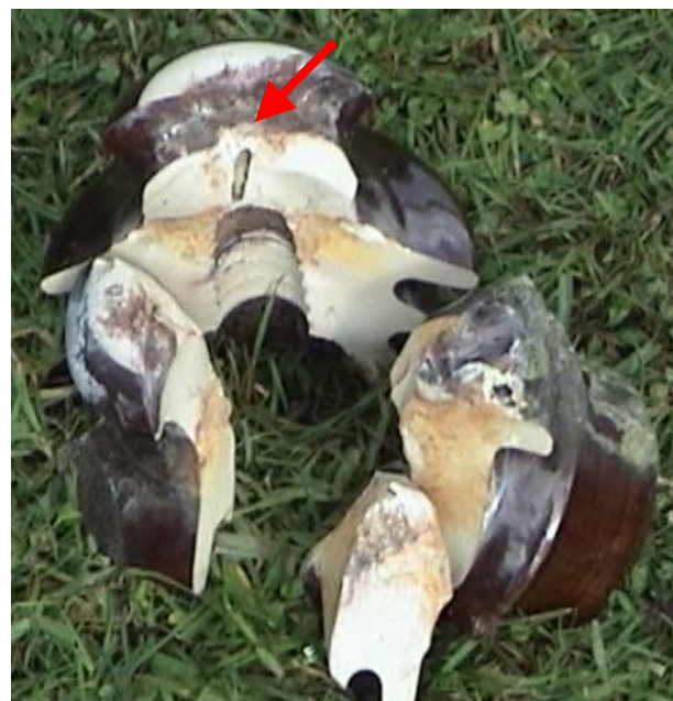
Figure 3: Insulator dissected to show pinhole.
