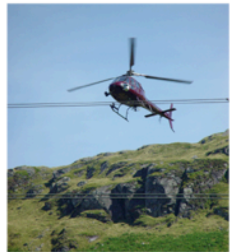
Helicopter overhead power line patrol using the DayCor II corona camera
