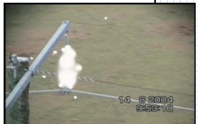
Airborne inspection: Strong discharge observed with the DayCor camera.
